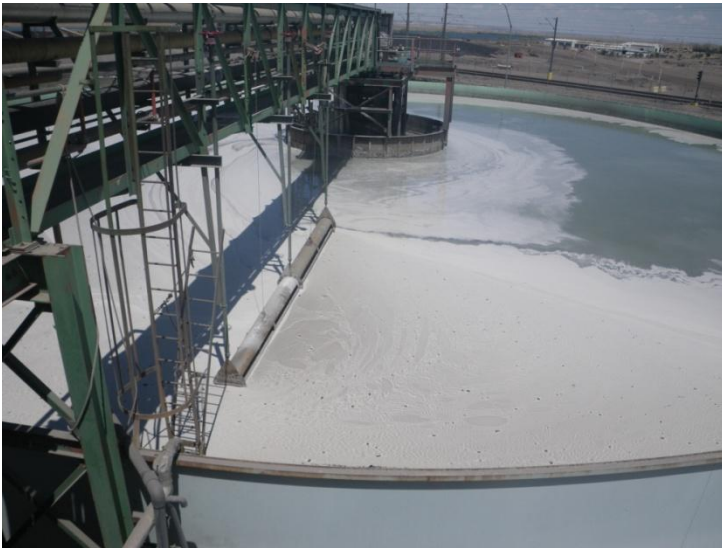
Figure 14: Thickeners from blowdown to be sent to fly ash ponds.
